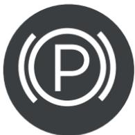
**The button in the center console to the left of the shifter is the emergency brake.** Push down to engage, flick up to disengage. If the car senses movement in "Park", it may automatically engage the e-brake. If this happens, it'll automatically remove it when you put the car in "D" or "L". Don't drive if this is showing on the top-right corner of the dashboard.
