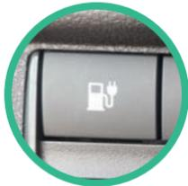
3. Push the button to the left of the steering wheel to open the charge door, located at the front of the car
